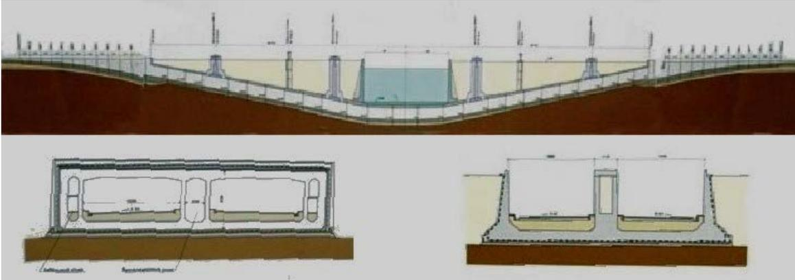
Figure 10: S1 Navigation Opening - tunnel sections
